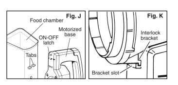
interlock bracket on the bottom of the slicing chute is not positioned in the bracket slot on the motorized base, (Fig K). Should the ON-OFF switch operate intermittently, check the position of the food chamber. Realign it so it is centered properly.
